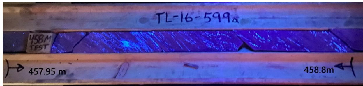
Figure 4: TL-16-599a: Scheelite veins, locally folded, hosted in altered (silicified, sericitized) clastic metasediments with arsenopyrite and pyrite; under UV light; returned 1.03% WO 3 and 5.31 g/t Au over a sample length of 1.0 m (458 to 459m) within the Simmons Shoot.
